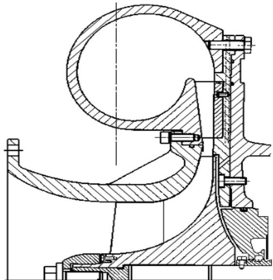
**Figure 1 Section of a high pressure turbocharger stage**
