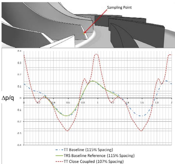
**Figure 14 Blade surface pressure at impeller exit**
