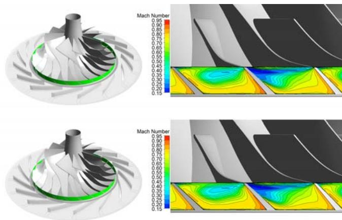
**Figure 13 Impeller exit relative Mach number distribution from steady state calculation**
